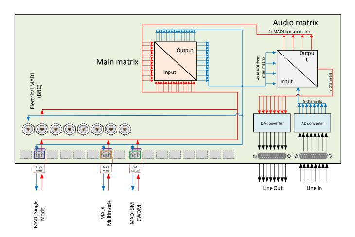
Channels of balanced analog line level audio are converted to digital audio. Via the 264x264 audio matrix the signals can be distributed to random channels of 4 MADI streams. Input sensitivity of each analog channel is configured to +18dBu or +24dBu individually.
